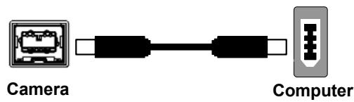
Figure 13: 9-pin to 6-pin FireWire (IEEE 1394) Port connection
