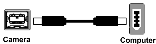
Figure 3: 9-pin to 6-pin FireWire (IEEE 1394) Port connection
