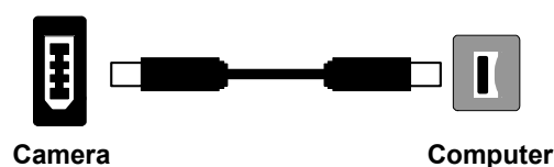
Figure 2— 6-pin to 4-pin FireWire (IEEE 1394) Port connection
